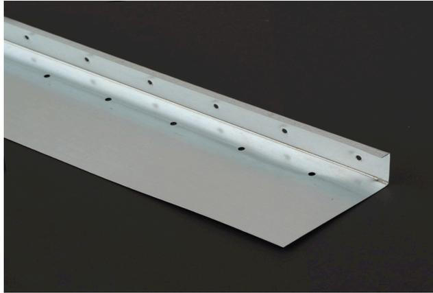
**The Niles No. 66N Long Flange/J-Weep comes standard with 3-1/2” flange and is intended for exterior applications with one & three coat stucco systems. Has a short 90 degree turn at the ground to neatly terminate plaster at the end of a wall or where it adjoins a dissimilar material.**
